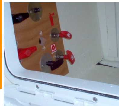
2: Inert gas projection lever
