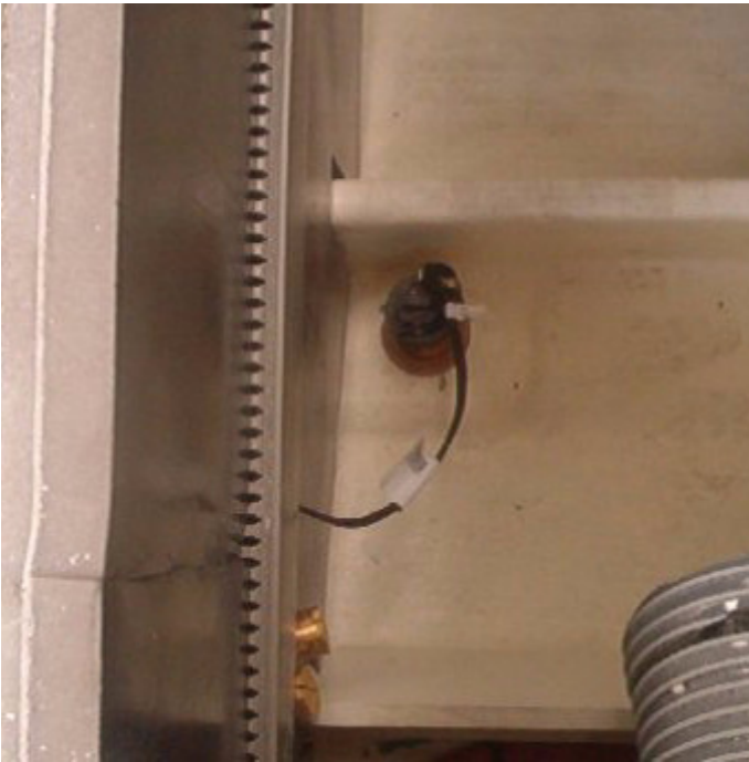
1 - Depth sounder - Log and speedometer Access through trapdoor in side cabin
