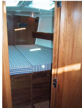
7. Unscrew the vertical panel of the locker under the berth.
