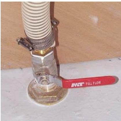
Thru-hull fitting **closed**
