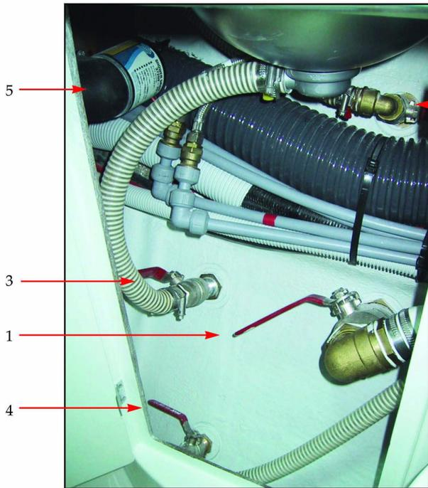
1. Thru-hull fitting with valve for heads draining
