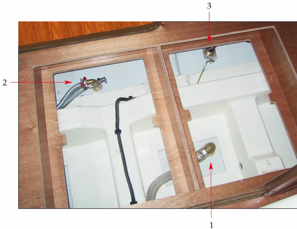
1. Thru-hull fitting with engine water inlet valve
