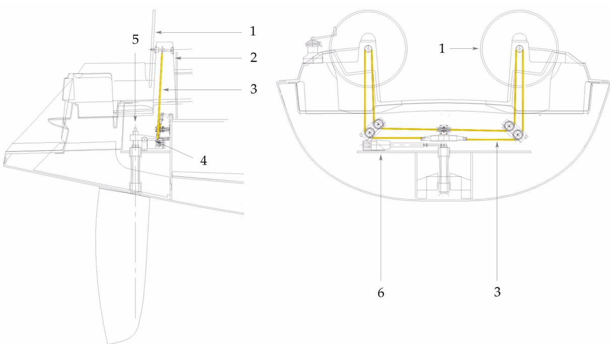
Access to the steering cables through the aft cockpit locker
