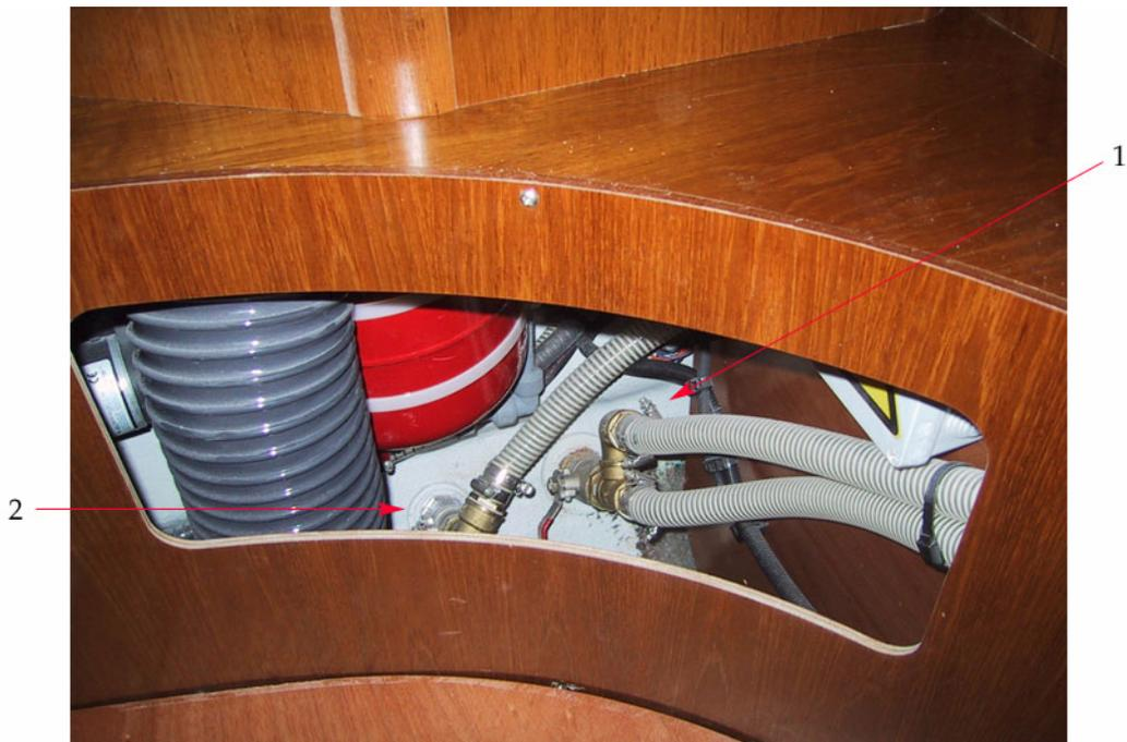
1. Thru-hull fitting with valve, draining of the sink
