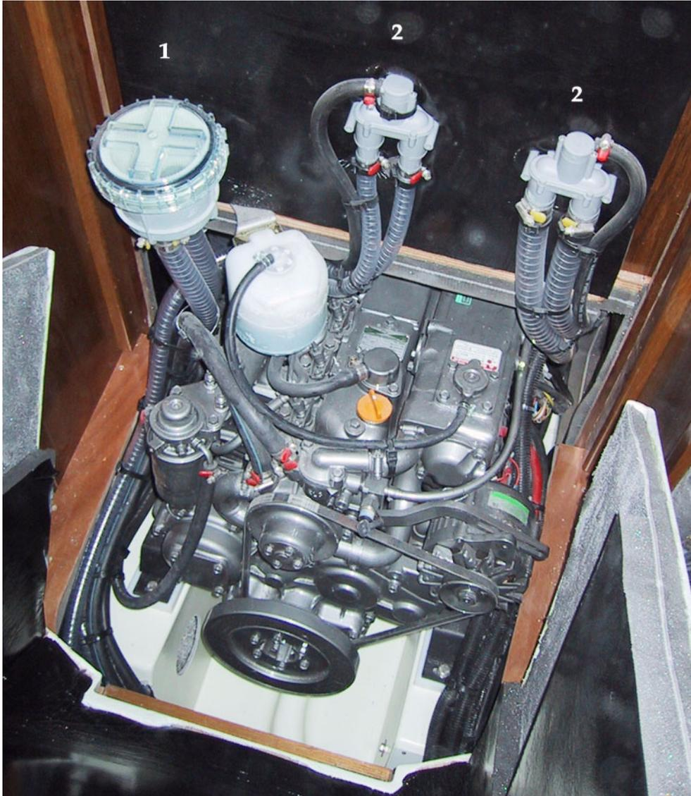
1. Filter for engine cooling water
