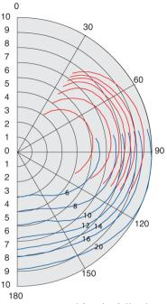
The tests were executed for the following rigging: mainsail, genoa stay sail, spinaker at 6, 8, 10, 12, 14, 16, 20 knots wind speed.
