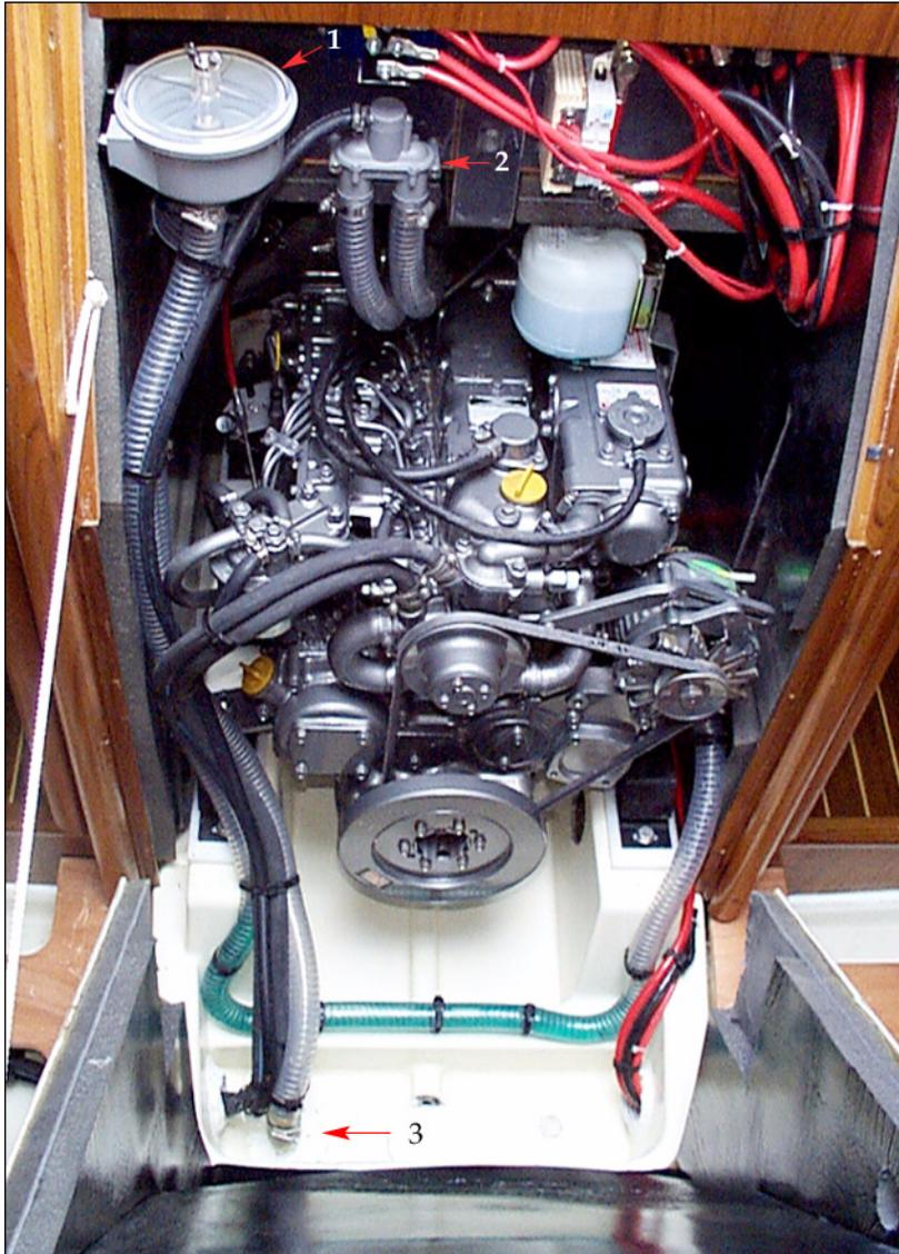
1. Filter for engine cooling water
