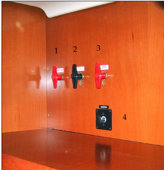
1. Battery switch + Engine
