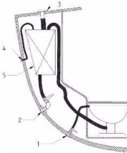
1. Heads water intake hose with a thru-hull fitting and a valve
