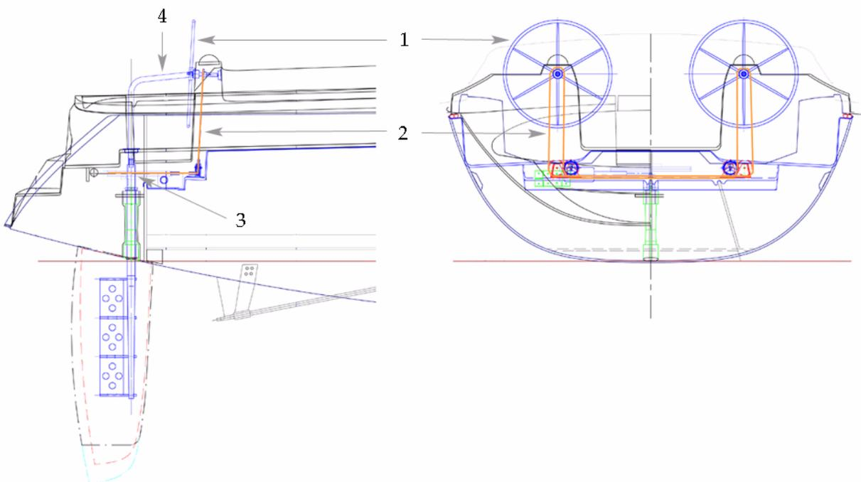
Access to the steering cables through aft cabin
